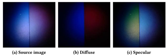
**Figure 1:** This figure shows in (a) a specularity on both a blue and a red planar object. (b) The diffuse component is extracted with polarizers. (c) Specular component is obtained by a subtraction operation (a) - (b). We observe in (c) an inconsistency of the specular component's color, which should have the same color on both surfaces (according to the dichromatic model).
